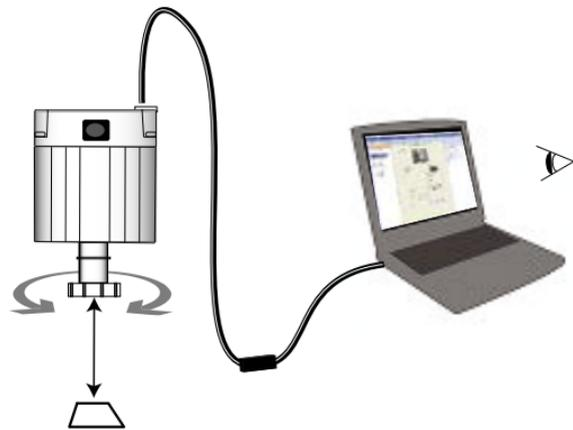
Adjust the lens focus while observing the image display in the Setup tool.
