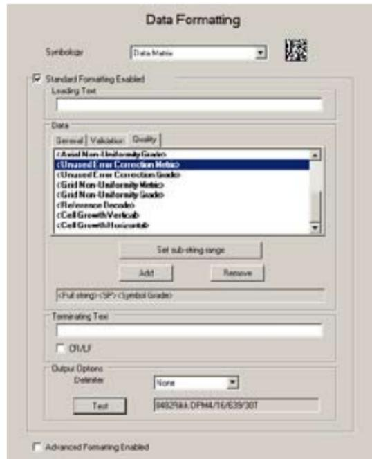
In addition to standard formatting, the DataMan Setup Tool supports the use of Perl-Style Regular Expression features in Advanced mode.
