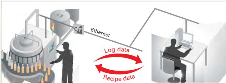
By accessing the CF/SDcard/USB storage of the Pro-face HMI main unit using file transfer, you can read or write log and recipe data.
