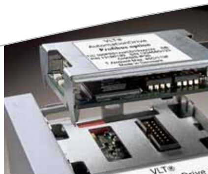
The fieldbus option ready to plug in beneath the front panel. It can be turned upside down if you'd rather have the cable on top.
