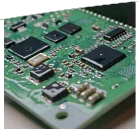
Coated control boards are available for harsh environments.
