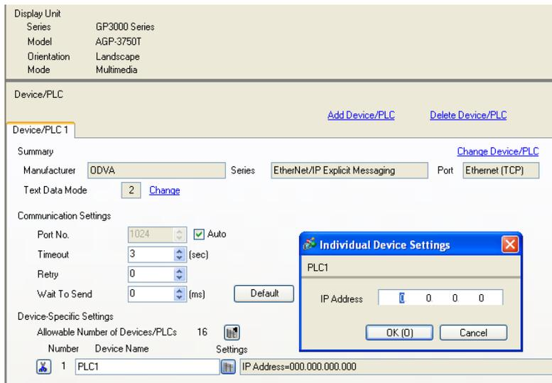
Enter the correct IP Address for the WAGO node and select OK
