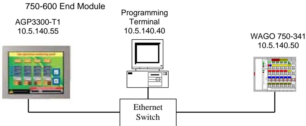
**NOTE:** This procedure assumes that the WAGO 750-341 contains a valid IP address and it is installed on a working network, along with the Proface HMI and GP-ProEX programming tool. If necessary, refer to WAGO's Application Note A202900 for assigning a static IP address to the WAGO 750-341.
