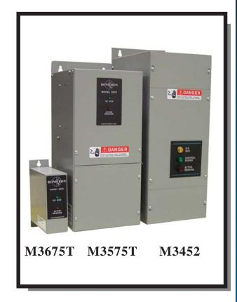
M3452 series modules are designed to be used with drives that have an inadequate or no internal braking transistor. They monitor the DC drive bus levels and control the IGBT power switch which connects the load across the bus. Standard models include fusing and are rated up to 600 Amps DC.
