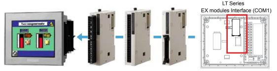
Up to three EX modules can be combine with LT Series to expand I/O requirements
