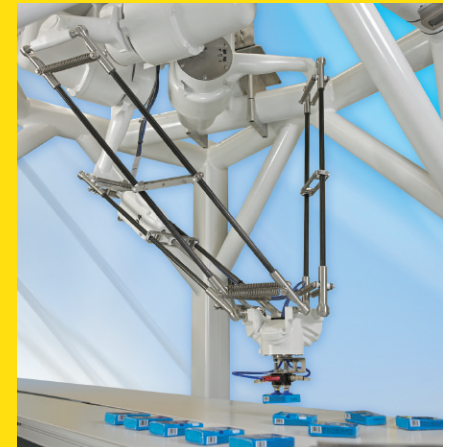
A single-axis wrist moves parts extremely fast
