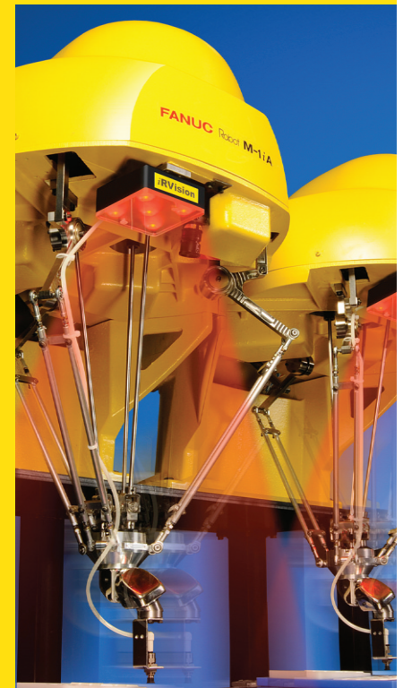
i RVision (built-in) for guidance and error proofing
